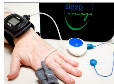
The Nonin WristOx (left) measures blood oxygen during sleep. The M1 recorder (right) measures the electrical activity of the heart.
